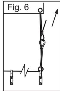
To tighten, pull loose end of rope through the Oval Compression Sleeve (Fig. 5). Stretch the bungee cord making sure all slack is taken out of the rope, crimp compression sleeve (Fig. 6). Be sure to keep flaps even on sides so Tie Down Ropes remain equal in length.
