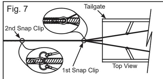
Flip the rope back on top of the tarp, making sure to hold the bungee at all times. The first snap clip is factory installed 5'-6" from the pullrod. Open the clip and enclose the rope. Weave the second clip through the main pullrope where the ends of the bungee cords meet the main pullrope. Make sure the rope is taught when clipped (Fig. 7).
