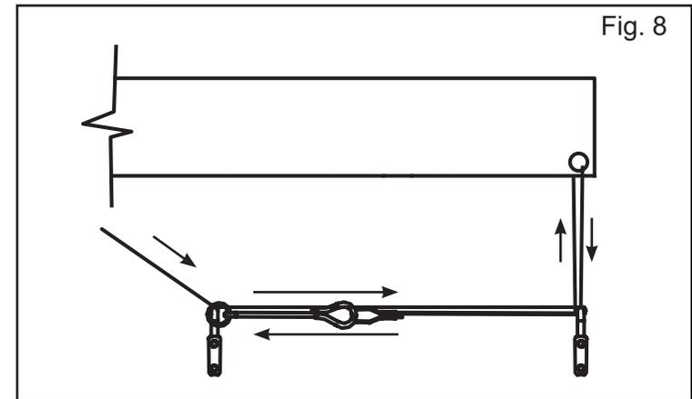
You may need extra rope to keep the side flap system ground operated. If your application requires extra rope, the slack needs to be taken up by attaching the end of the bungee cord to an alternate hook (Fig. 8).
