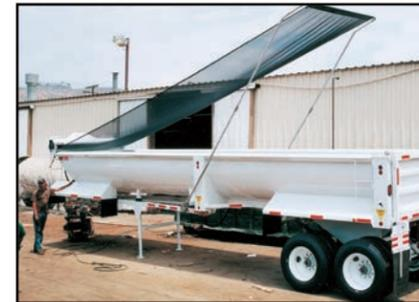
Electric Arm System with Heavy Duty Mesh
